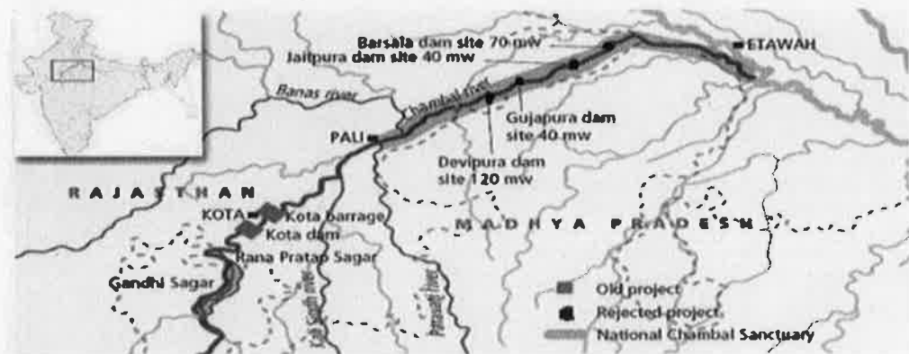
Map 8.1.3 Showing the Chambal River, National Chambal Sanctuary and Kota dam and barrage – flood in the Chambal River valley areas occurs when Chambal River overflows due to release of excess water into the river by the Kota barrage
